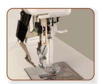
Acufeed: Layered Fabric Feeding System It perfectly guides your fabric from both the top and the bottom. Only Janome truly integrates a built-in walking foot with a unique sevenpoint feed dog system.
