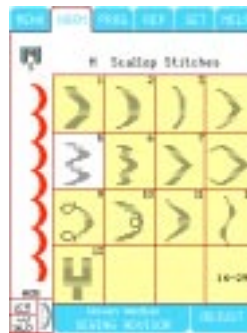
MENU H: SCALLOP -27 styles of scallop stitches up to 25 mm wide. Program them for 35 mm width.
