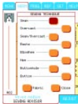
SEWING ADVISOR TECHNIQUE -Touch desired sewing technique. Designer I sets best stitch, width, length, tension, sewing speed and presser foot pressure instantly.
